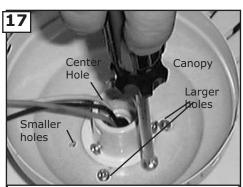
Place canopy on top of the fan motor allowing the yoke to pass through the large hole in the center of the canopy. Align the 3 larger holes around the center hole with the 3 screws already installed in the fan. Install 3 flush mount screws provided into smaller holes and tighten securely.
